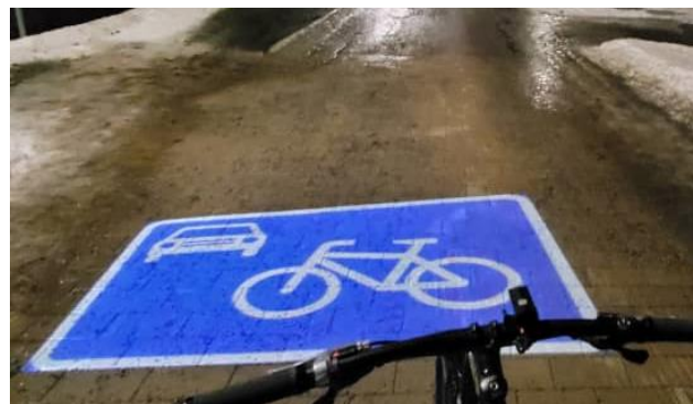
Figure 30. Traffic signs get projected onto road surface to indicate a shared space between cars and cyclists in Vaasa, Finland (Image Credit: Arup)
